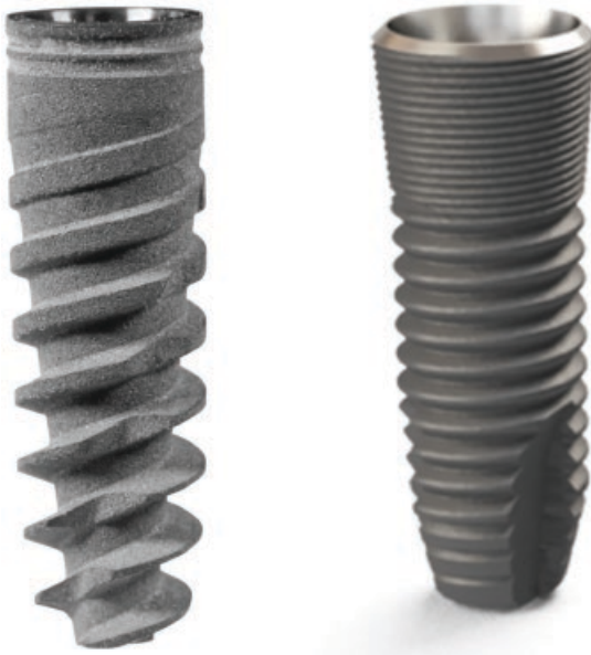
Figure 2.10 Shows the progressive change in an implant thread design: The implant on the left shows the change in the depth and pitch of the threads, and the implant on the right shows the microthreads at the top aimed at improving the contact with the coronal bone.
