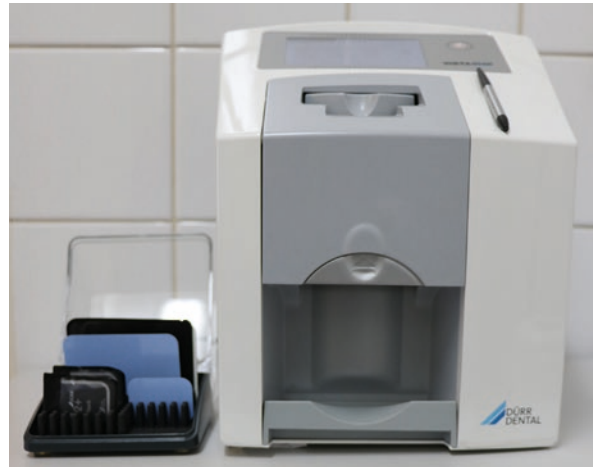
Fig. 2.4 Laser scanner for intraoral indirect digital radiography
