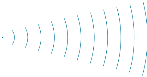
Figure 1-4. The curvature of wavefronts becomes less as the distance from the point source increases. They are arcs of a circle whose center is the point source. At infinity, the wavefronts are flat.
